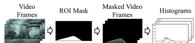
Fig. 9. Flow diagram of the process for extracting the ROI histograms from each image in a time-series video.
