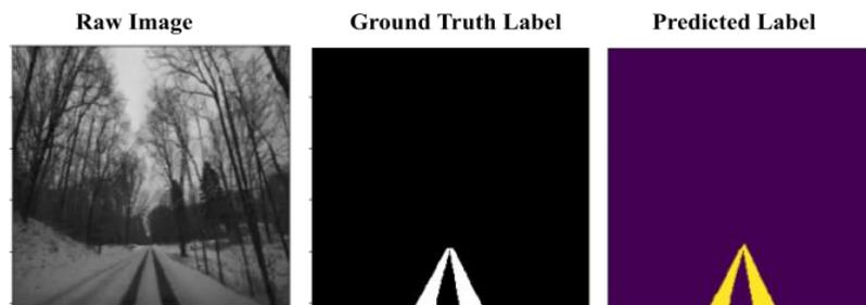
**Figure 5. CNN output (The raw image is on the left, the labeled segmentation mask is in the middle, and the predicted segmentation mask from the CNN is on the right)**
